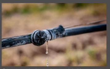
Drip emitter with calcium carbonate scale buildup, suggesting the emitter is plugging.
